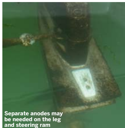
Even shaftdrive GRP boats need anodes to protect their stern gear
